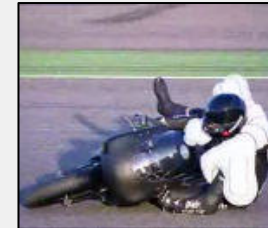
Side crash detection and motorcycle airbag: 100 - 480 g
