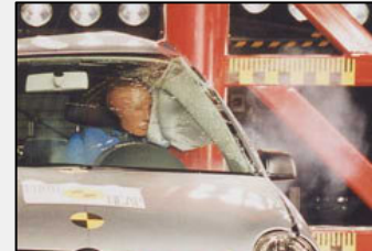
Side crash detection and motorcycle airbag: 100 - 480 g
